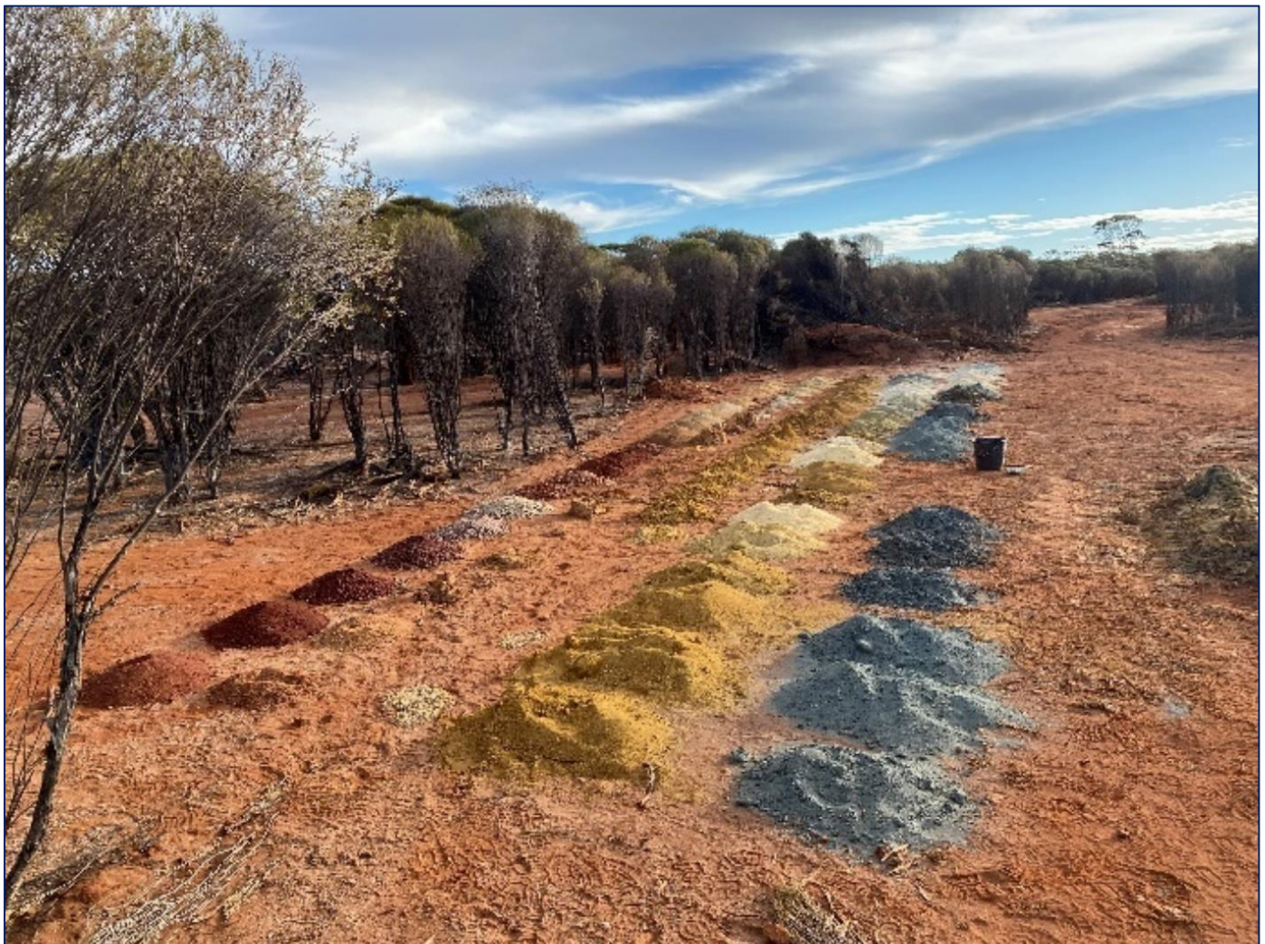
Figure 10 – RC drilling sample piles at Olga Rocks Project showing grey and dark grey mafic to ultramafic lithologies
