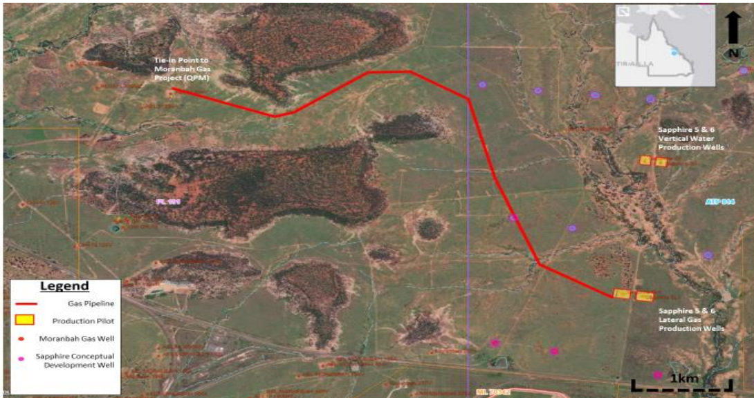
Figure 2: Provisional pipeline route for tie into QPME's Moranbah Gas Project low pressure network
