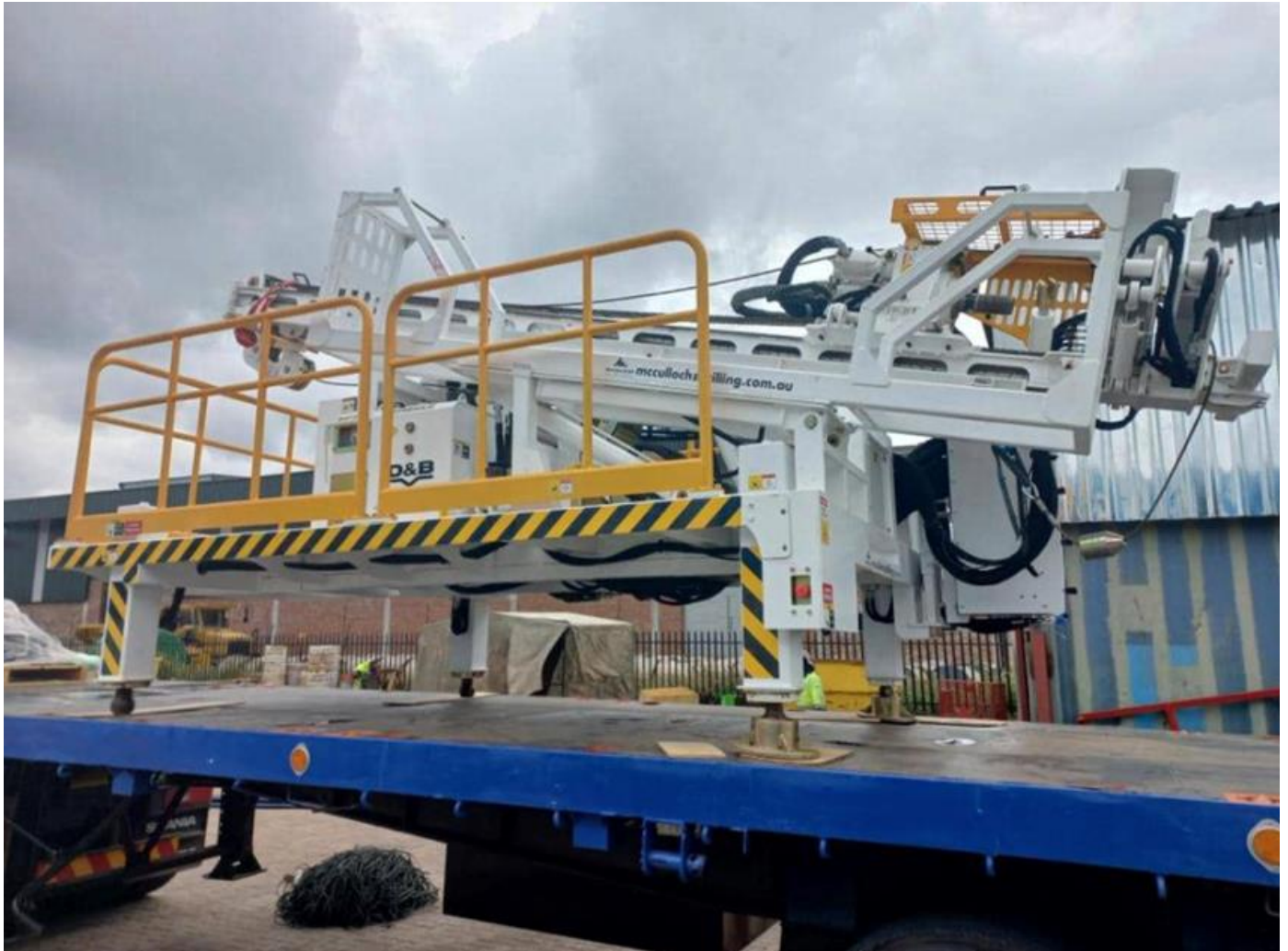
Figure 9: Mitchell's AC and RC slimline drill rig which is being used in combination with conventional RC to complete the 10,000m drill program at NCP and KITW, currently underway.
