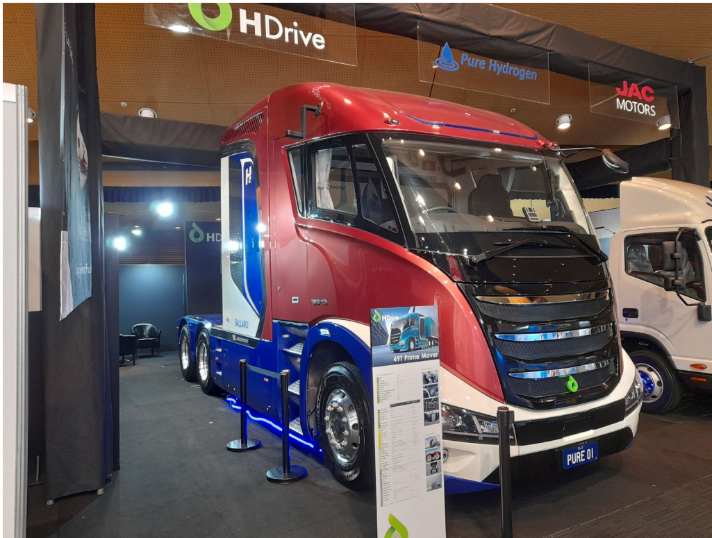
Image 3: “The Taurus”, a 220KW 6 x 4 hydrogen fuel-cell Prime Mover on display at the Brisbane Truck Show in May 2023
