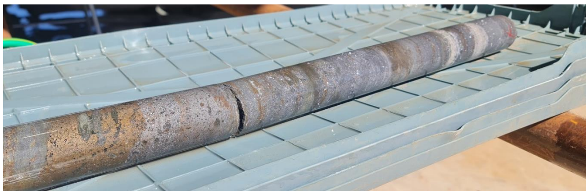
[Figure 2] MRN23008 - Core stick of semi-massive galena matrix breccia from the Western Horizon around 322m down hole
