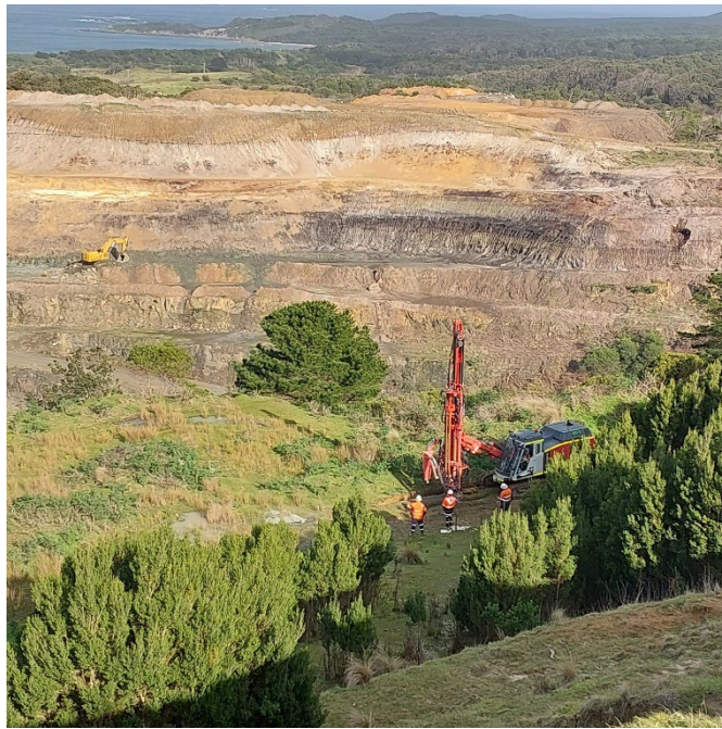
Figure 5 - Commencement of drilling on the north cut back of the Dolphin open cut.
