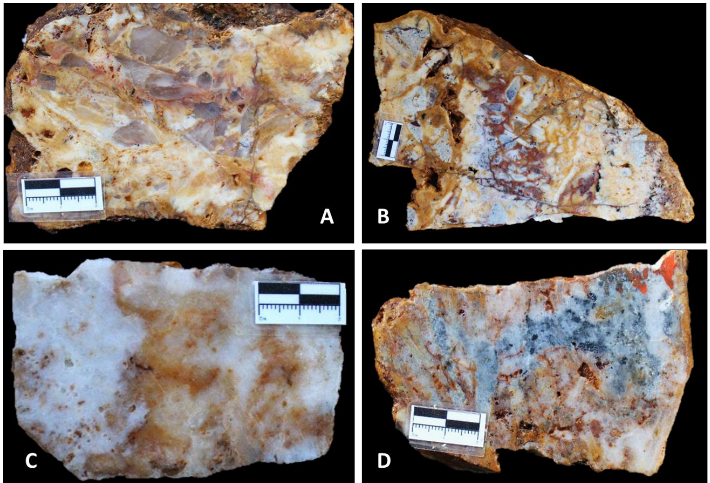
Figure 11: Photos of samples taken from the Kareung Reuboh quartz veins. A) grab sample of quartz breccia from 2m wide vein. Oxidized with minor disseminated pyrite. Assay 4 g/t Au, 0.9 g/t Ag, B) grab sample of oxidized quartz breccia from 2m wide vein. Disseminated pyrite. Assay 19.41g/t Au ,12.8 g/t Ag, C) chip sample of oxidized massive crystalline quartz vein, minor colloform bands present, disseminated pyrite (2%). Assay 16.12 g/t Au, 15.9 g/t Ag, D) chip sample of quartz breccia with disseminated black sulfides in less oxidized part of the sample. Abundant pyrite. Assay 98 g/t Au, 77 g/t Ag.
