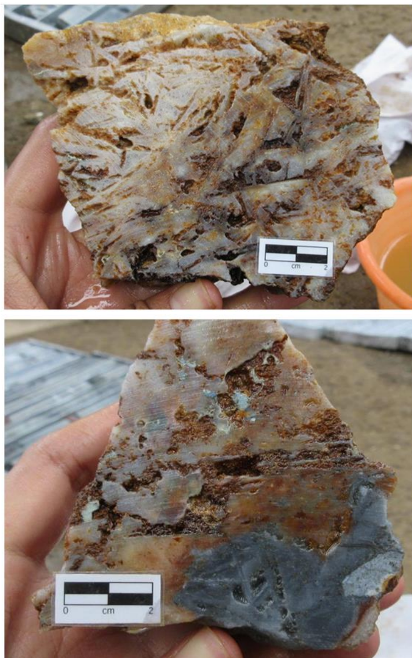
Figure 12: Grab samples collected from the Aloe Rek prospect area. TOP: quartz vein sample taken from artisanal mining pit, at 20m depth. Vein was 3-5m wide, crystalline quartz with bladed texture, oxidized. Assay of 14.9 g/t Au, 22.1 g/t Ag. BOTTOM: grab sample of quartz vein, taken at 20m depth from an artisanal mining shaft. Sample contains abundant arsenopyrite in lower right part of the quartz. Assay of 9.1 g/t Au, 20.5 g/t Ag
