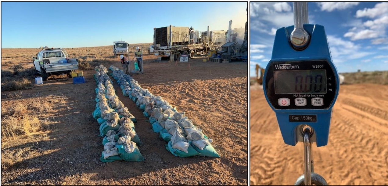
Figure 6a: RC samples laid out in rows of 30 x 1m sample piles (1 pile = primary, secondary & bulk samples). Note the weighing rig in use near the end of the second row of samples. At right: Wedderburn digital scale used on weighing rig.
