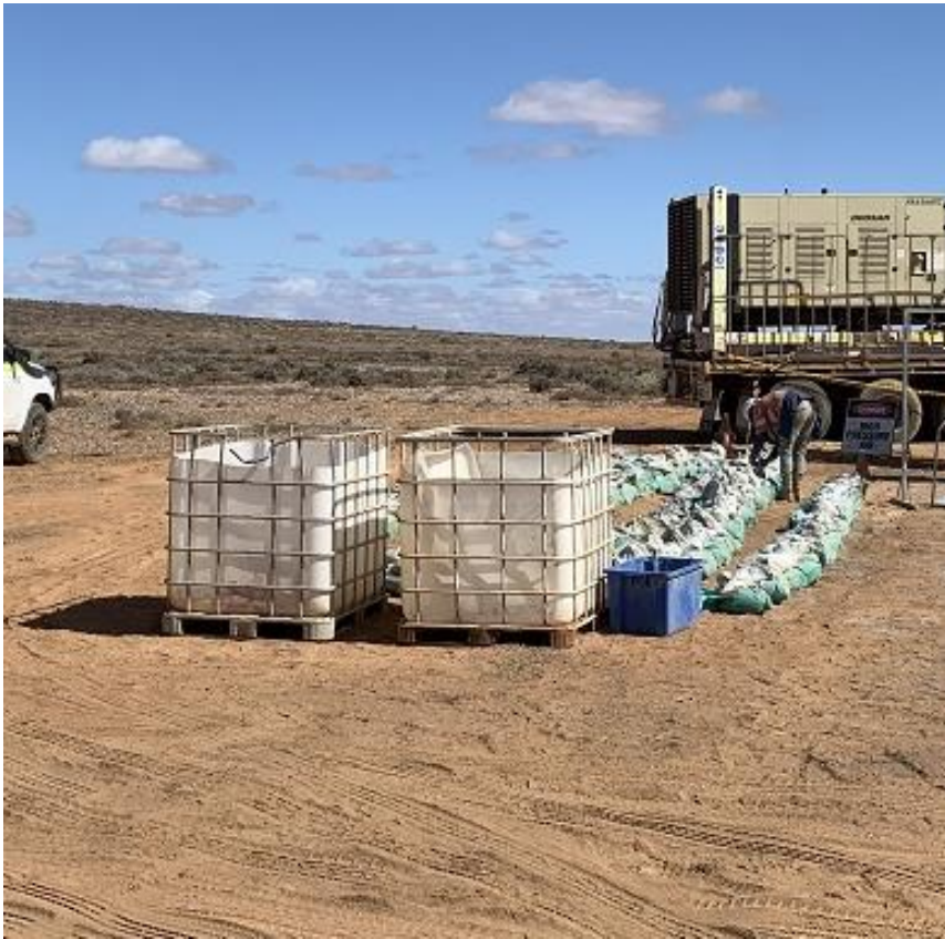
Figure 7: IBC containers at hole site (with top cut-off as lids) lined up ready to load samples (the lids are inside the containers and will be screwed on before transportation).
