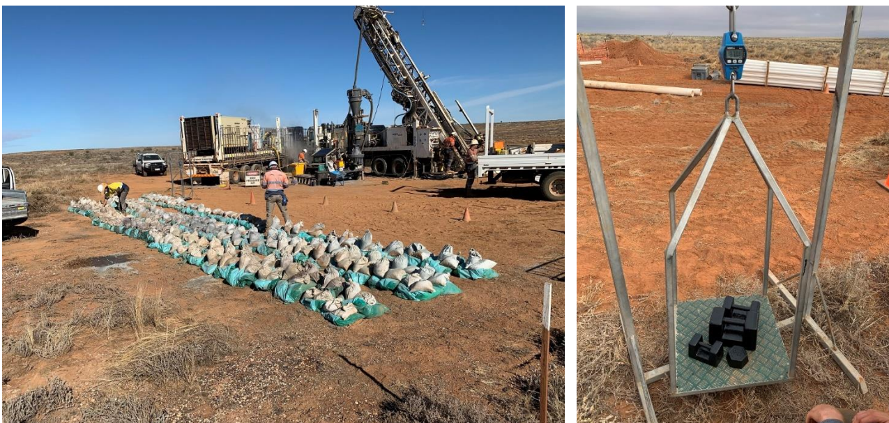
Figure 6b: Magnetic susceptibility measurements being taken on completion of sampling. Samples laid out in rows of 30 x 1m samples. At right: weighing rig being calibrated against the full suite of standard weights (37kg).
