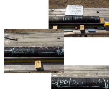
The next phase of the programme now commences with analysis of the core samples taken during drilling which have been delivered to the laboratory. The photos above show some of the core from hole BCP4.
