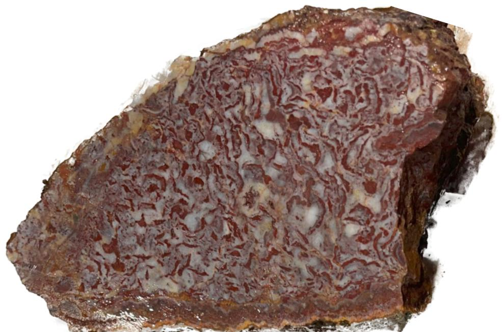
**Figure 5.** Sample 7207: 1.79g/t Au, 3.67g/t Ag and 72.5ppm Sb
