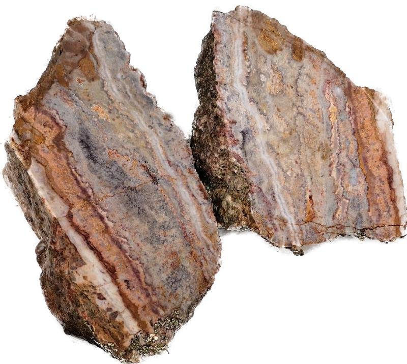
**Figure 8.** Sample 7314: 2.18g/t Au, 11.75g/t Ag, and 64.9ppm Sb
