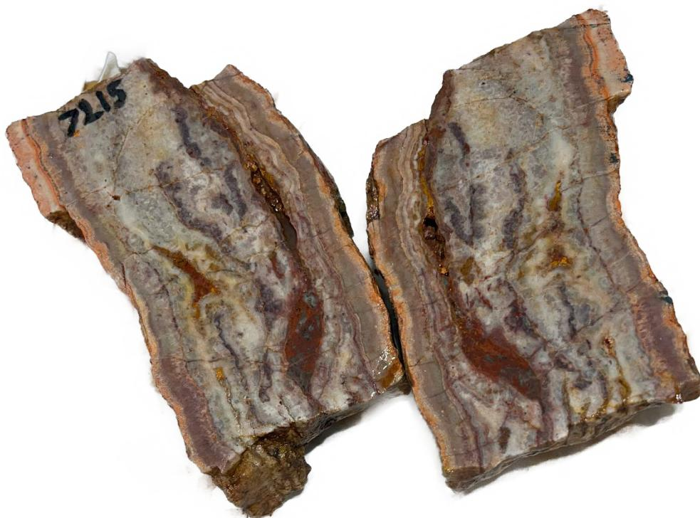
**Figure 10.** Sample 7215: 1.32g/t Au, 2.45g/t Ag, and 111.5ppm Sb
