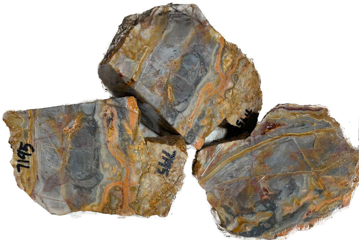
**Figure 7.** Sample 7195: 2.66g/t Au, 1.54g/t Ag, and 159ppm Sb
