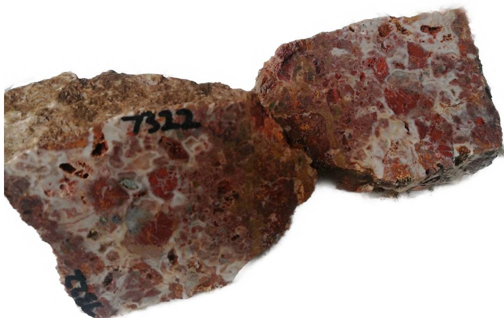
**Figure 6.** Sample 7322: 3.86g/t Au, 4.02g/t Ag, and 76ppm Sb
