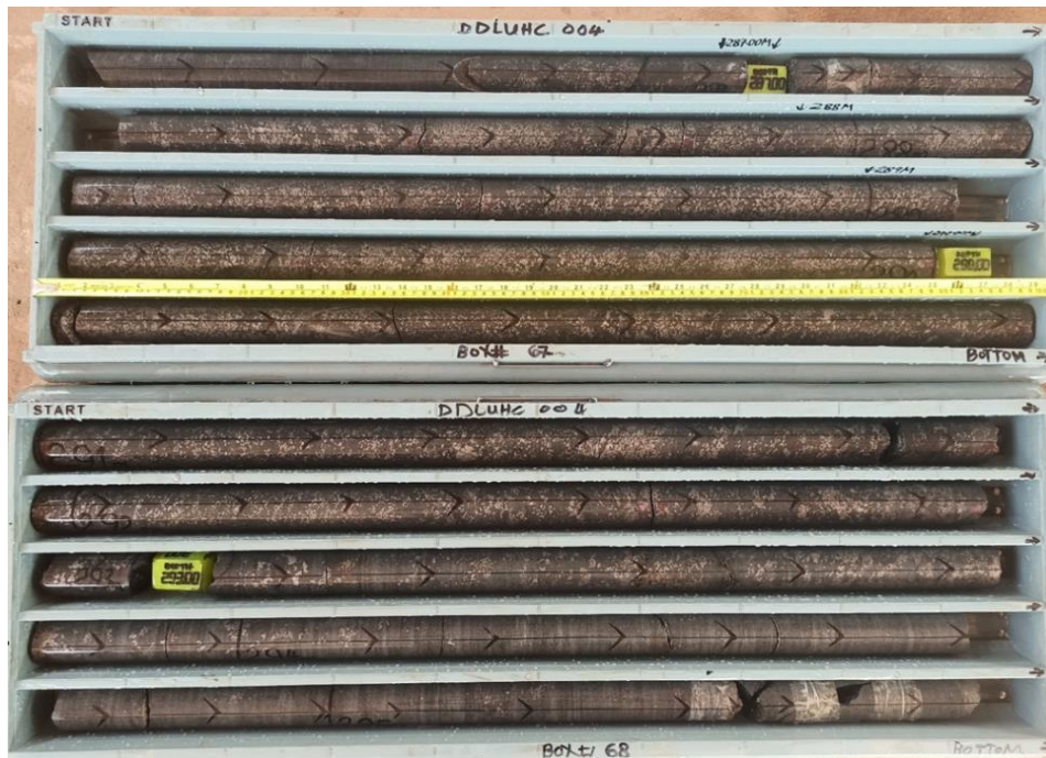
Figure 3: Photograph of Semi-massive sulphides from 286.70m to 294.20m
