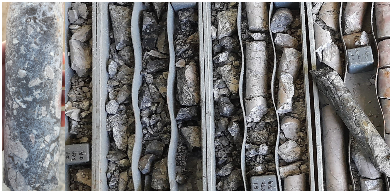
Secondary chalcocite mineralization (black mineral) in volcanic rocks
