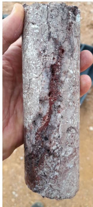
Porphyry B-veins and breccias with abundant iron-oxides (after sulphides) preserved in oxide gold zone
