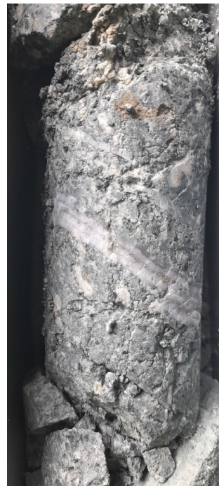
Porphyry B-veins and breccias with abundant iron-oxides (after sulphides) preserved in oxide gold zone
