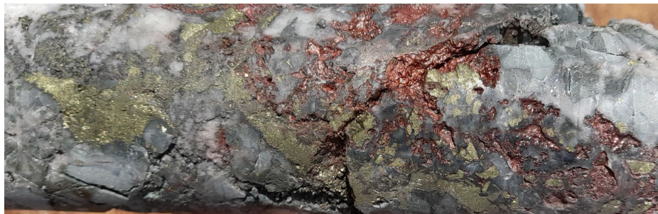
Chalcopyrite veining with native copper at the oxide-sulphide boundary
