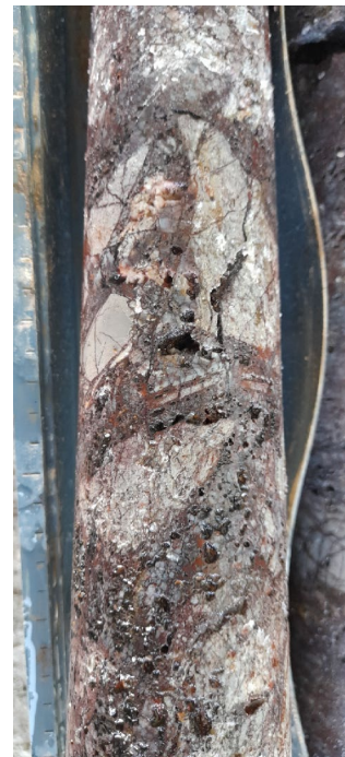
Porphyry B-veins and breccias with abundant iron-oxides (after sulphides) preserved in oxide gold zone
