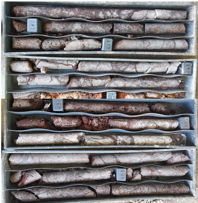
Oxide gold zone in drillcore (iron-oxide veining and stockworks after sulphides)
