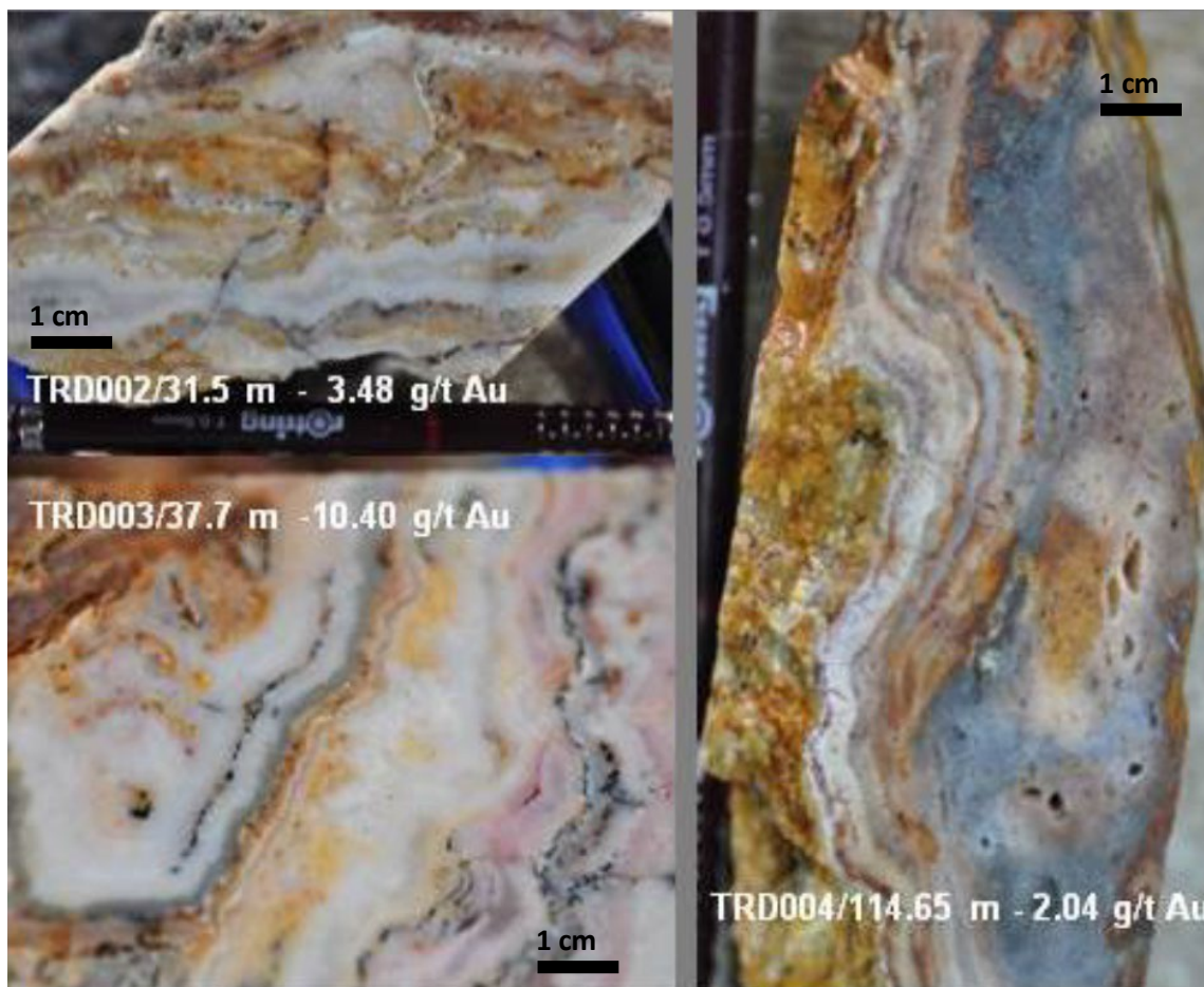
Figure 5: Core specimens of drillholes in the West Sentul vein system showing examples of crustiform-colloform quartz- sulphide textures that occur. These are characteristic of ginguro-type bands that are often associated with high-grades of gold-silver in such vein systems. The gold grades indicated are recorded in historical assay reports. While the Company has confirmed the presence of such textures it has not conducted any additional core sampling to confirm reported grades.
