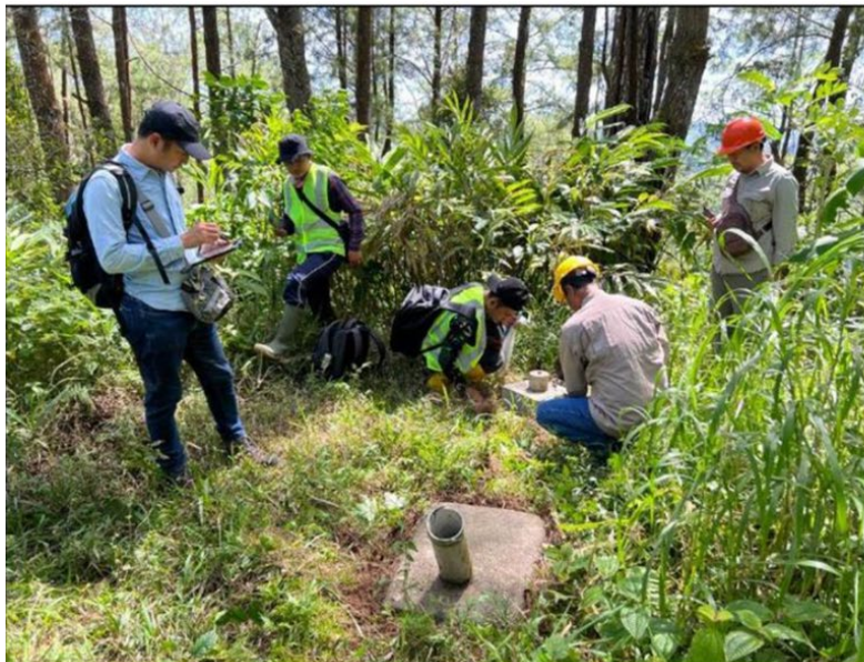
Photo 1 and 2: Detailed mapping in the area of quartz-sulphide breccia occurrence. Left- FEG field team confirming the locations of previous drillhole TRD025. Right- new exposure of quartz breccia about 2m wide about 200m south of the breccia intersected by previous drilling.
