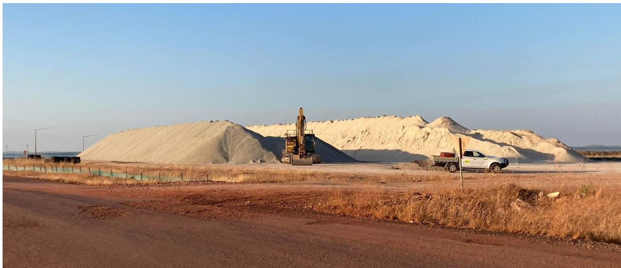
Fines and Spodumene Concentrate stockpiles awaiting shipment at Darwin Port
