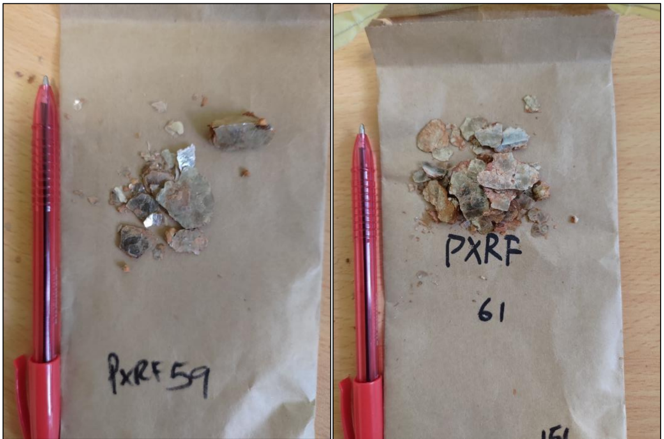
Figure 4 – Examples of muscovite samples collected from pegmatite outcrop. Portable XRF allows for quick field evaluation of the pegmatite’s LCT potential, based on the key geochemical indicators, K, Rb, Cs, Ta, Sn, Nb.
