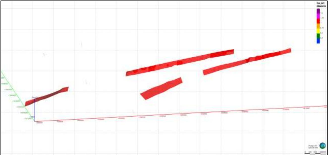
Figure 8: Northeast view of High-grade Mineralised domains (Cu % > 0.5).
