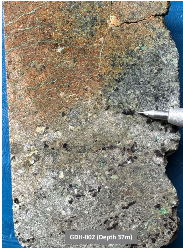
Figure 6: Fine-grained diorite with Sericite, illite & Anhydrite alteration, disseminated secondary chalcocite. (GDH-002 at 37m)
