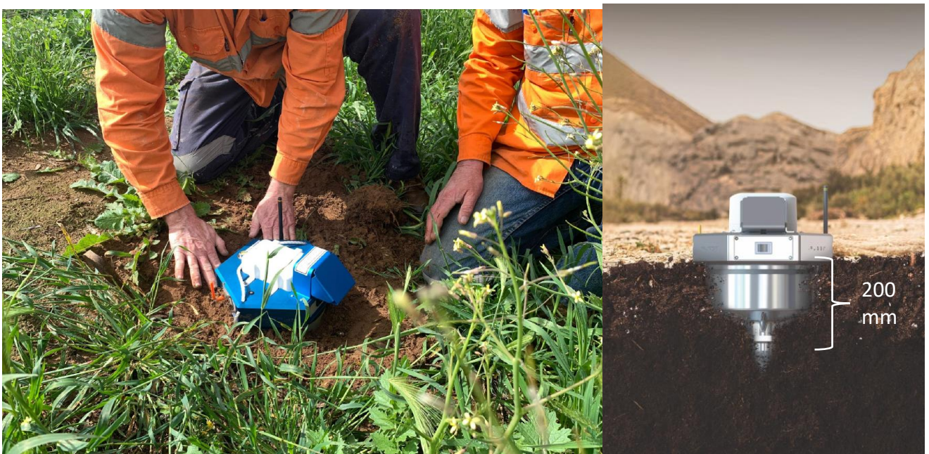
Figure 3: Exosphere used by Fleet Space® for ANT surveying.
