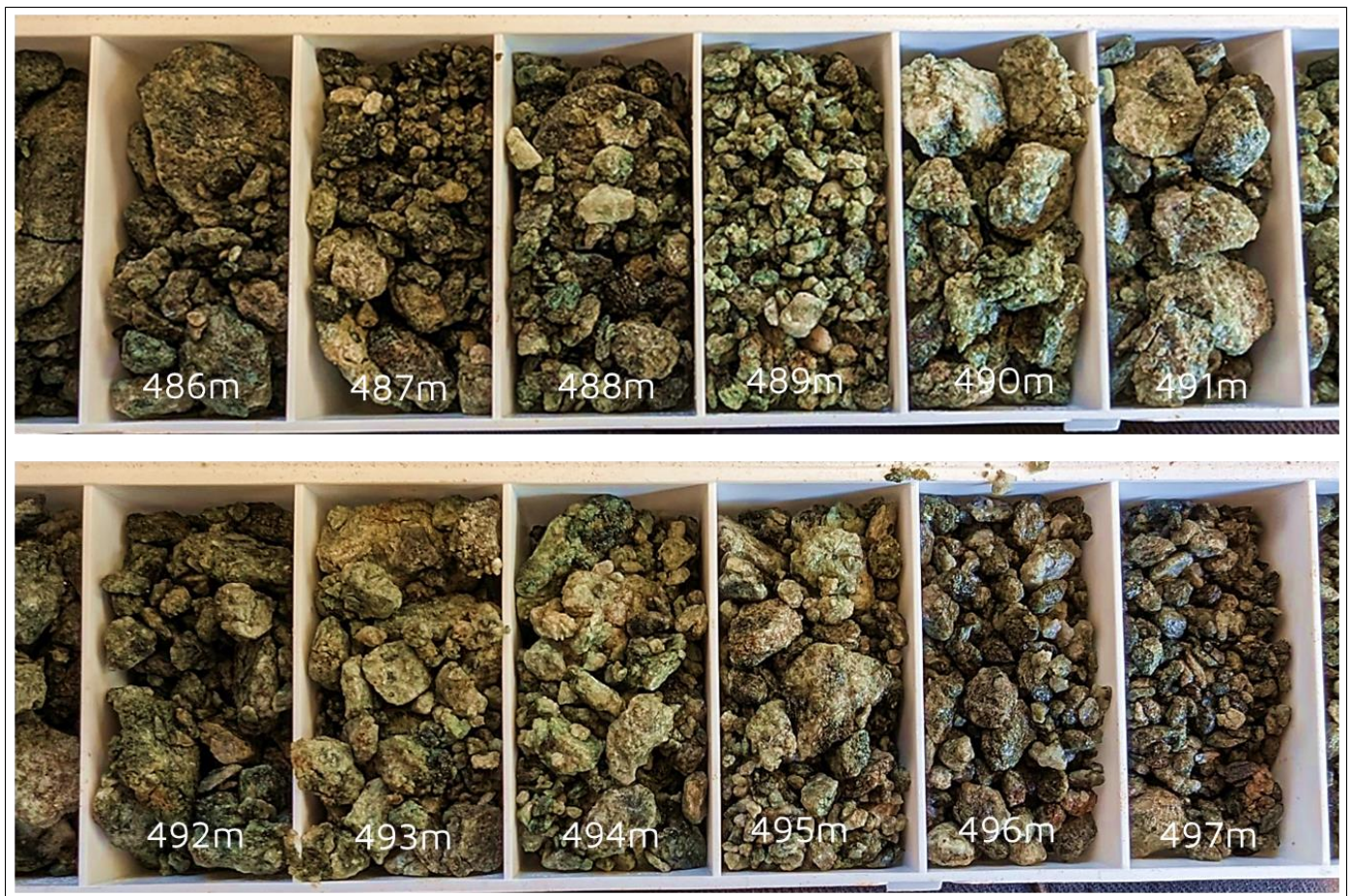
Figure 3. RC chips in WDNRC002 (486m to 497m) displaying a zone of intense biotite-actinolite altered komatiite with abundant quartz-carbonate alteration and highly anomalous Arsenic and Antimony.
