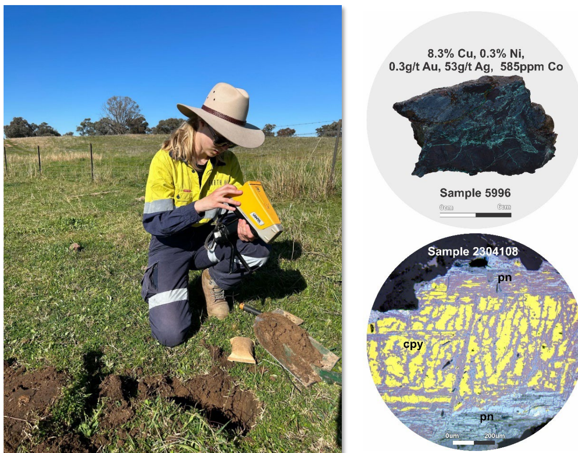
Figure 3: Earth AI field team conducting soil sampling at Fontenoy (left), and rock sample 5996 (top right), and nickel sulphides (pn - pentlandite), copper sulphides (cpy - chalcopyrite) confirmed in serpentinite/gabbro through SEM and petrographic analysis (bottom right) i .
