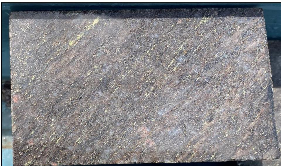
Figure 4. Visible chalcopyrite mineralisation developed within foliation in a metamorphosed quartz diorite porphyry intrusion. Core sample taken from CCDD001, 57m.
