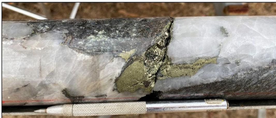
Figure 9. Quartz diorite hosting a massive quartz vein with chalcopyrite and pyrite mineralisation, with biotite and minor chlorite and epidote alteration also present (CCDD001, 67m).
