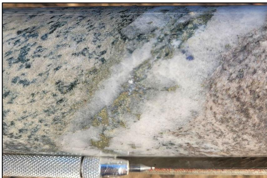
Figure 6. Mineralised (chalcopyrite-pyrite-molybdenite) contact between tonalite and quartz diorite (CCDD006, 263.7m).
