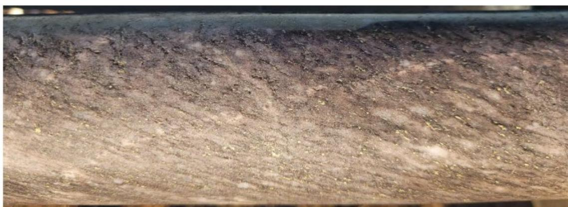
Figure 7. Quartz diorite porphyry with quartz eyes, showing strong secondary silica and biotite alteration and strong chalcopyrite mineralisation along the foliation (CCDD003, 140.5m).
