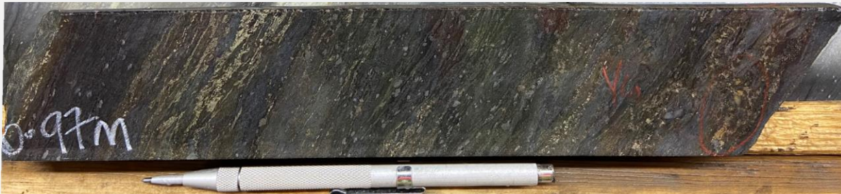
Foliated basalt with sulphide-magnetite replacement from MMTP with high-grade gold mineralisation
