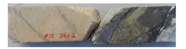
Downhole contact of argillised dyke with adjacent contact of semi-massive sulphide infill. CAE hole# 18, 361.2m. Interval 361m-362m: 1m @ 10.8 g/t Au ,0.88% Cu,40 g/t Ag, 6.5% S...
