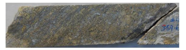
Very high grade gold section of semi-massive sulphide infill alongside contact of unusual argillised dyke cutting breccia. CAE hole# 18, 359.6m . Interval 359m-360m : 1m @ 96.2g/t Au ,1.46% Cu, 123 g/t Ag, 14.8% S, elevated Bi,Pb,Sb.
