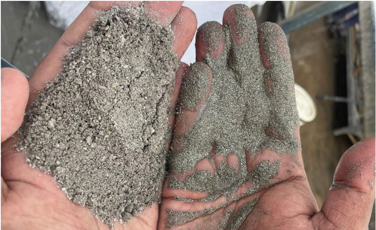
A total of 4,200t of ore was processed to produce 680t of wet concentrate (typical moisture 5–10%). A further 800–1,000t of ore remains for optimisation studies in the future. Operations were held over 65 days with the longest run of over 100 hours recorded. Mass recovery of ~17–20% was consistently achieved, with an average concentrate grade of 4,434 ppm Co (see Figure 6).
