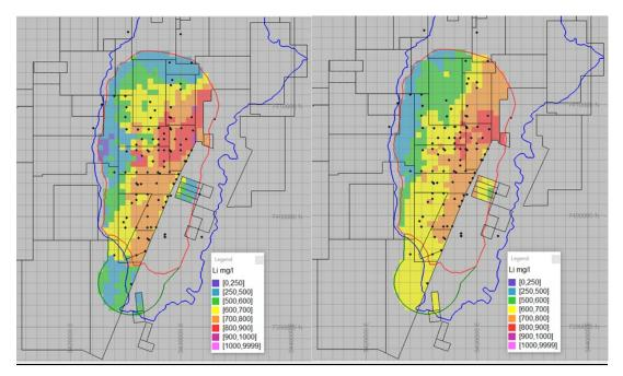
Figure 6: Lithium grades (mg/L) at 100 m (left) and 250 m below surface (right.)
