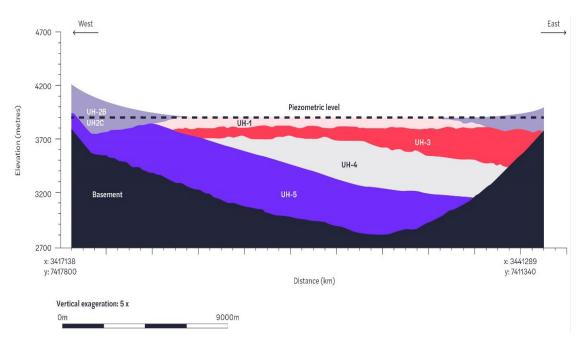
Figure 4: Geological model of the Olaroz salar looking north through the northern part of the basin
