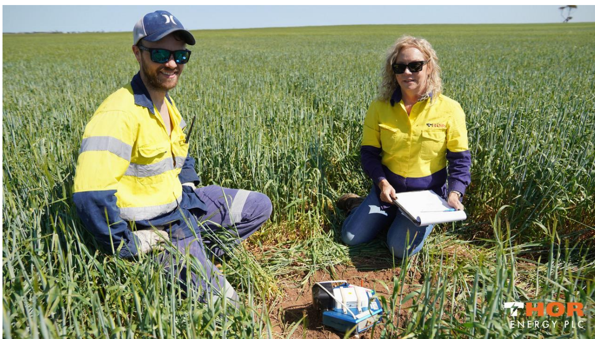
Photo 1: Deployment of Exosphere by Fleet® geodes for ANT Surveys, at Alford East Project
