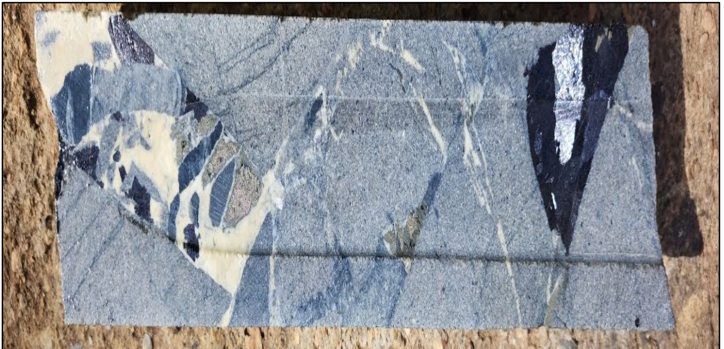
Figure 10: Breccia showing carbonate infill with sphalerite and pyrite mineralisation in MPD005 @ 260.2 metres
