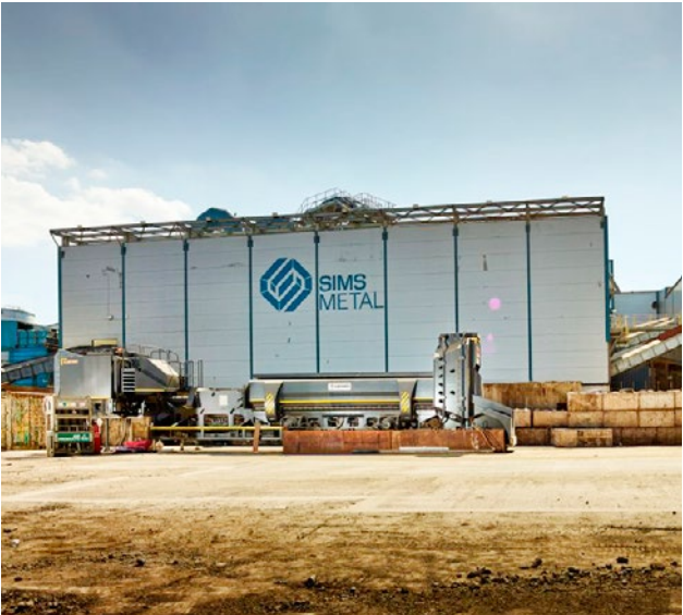
Electric shear installed at Avonmouth, UK, in front of acoustic baffle to contain noise from shredder operations.
