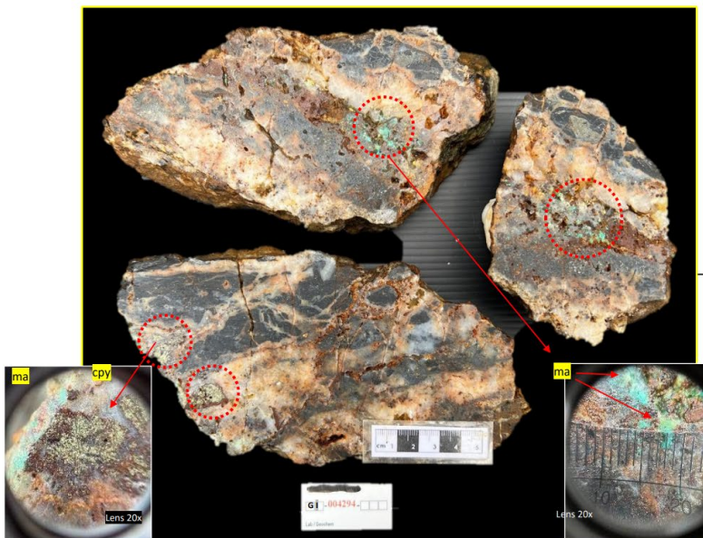
Figure 6: ABOVE – (GI004294); Quartz breccia vein, milky white to grey brown, weak-mod weathered, moderate lim-hem ox in fracture, breccia texture w/ VAN(?) as clast, qtz chalcedonic-xtln in cemented, massive, minor vugy texture, strong silica altered, 10-15% py diss, 1-2% cpy-ma blebs in qvn, wide +/-3m observe, w/ strike N 80°E/56°S & DD 185°/56°S. Assays returned 1.649 ppm au and 8,436 ppm Cu. RIGHT – Map showing location of sample.
