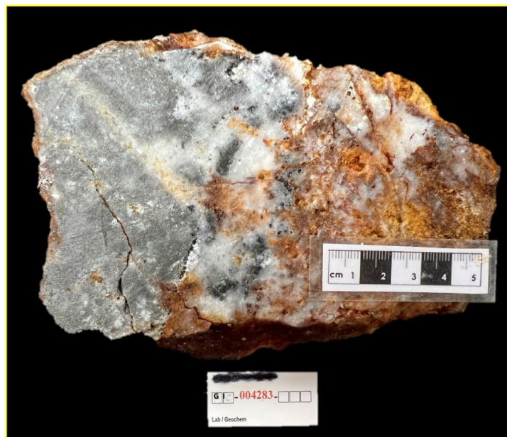
Figure 11: ABOVE – (GI004283); Quartz breccia vein, white, grey brown, weak-moderate weathered, mod-strong lim-hem ox in fracture, breccia text w/ andesite clast, qtz xtn vein in matrix, strong silica alt, minor vuggy & drussy text, 3-5% py diss, spotted <1% achantite(?), w/ 2m wide, undefined the direction. Assays returned 0.443 ppm Au and 448 ppm Cu. RIGHT – Map showing location of sample.
