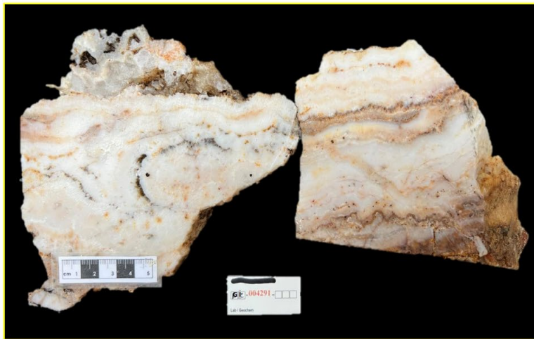
Figure 5: ABOVE – (GI004291); Quartz vein, milky white, weak lim-hem-Mn ox in fracture, qtz chalcedonic-xtln vn, massive to banded, minor vugy fill Mn ox, strong silica altered, trace py to 1% py spotted, wide +/-10m (top ridge), trend direction N 50-60E/80SE, DD 130-140/80SE. Assays returned 1.519 ppm Au and 20 ppm Cu. RIGHT – Map showing location of sample.
