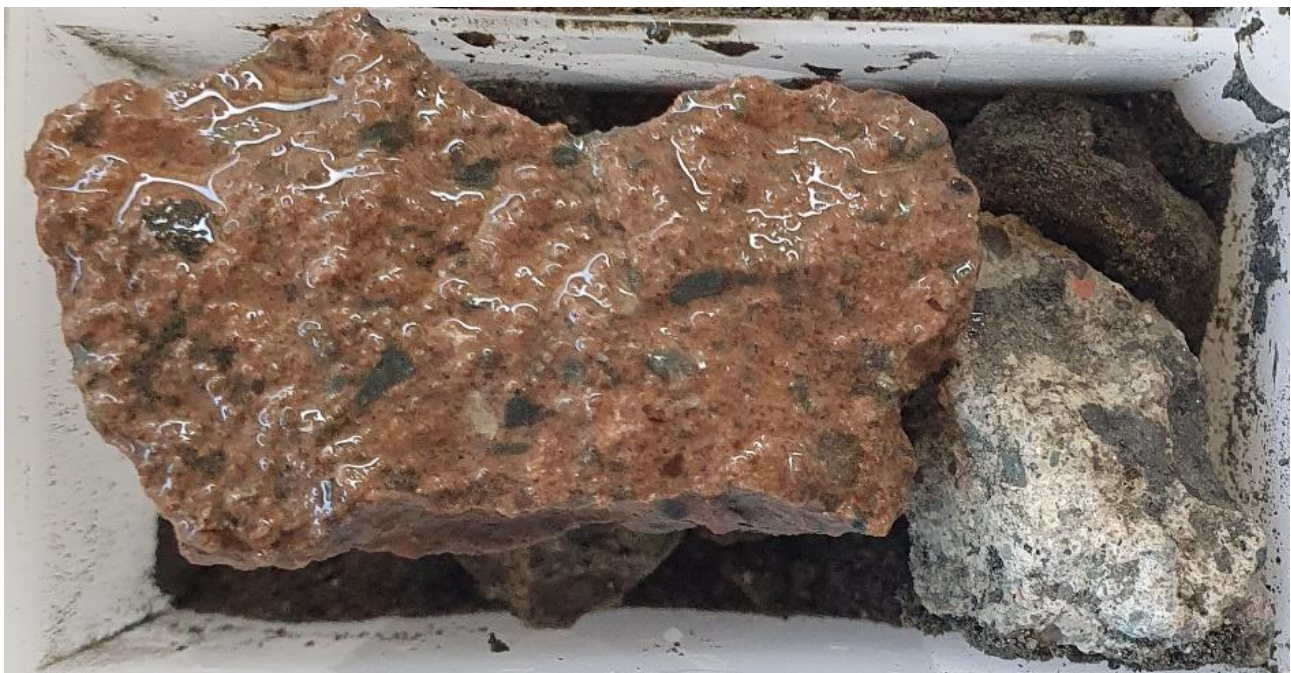
Figure 3: Quartz K-spar porphyry breccia chips at the base of NBG011. Large wet fragment ~15mm long.
