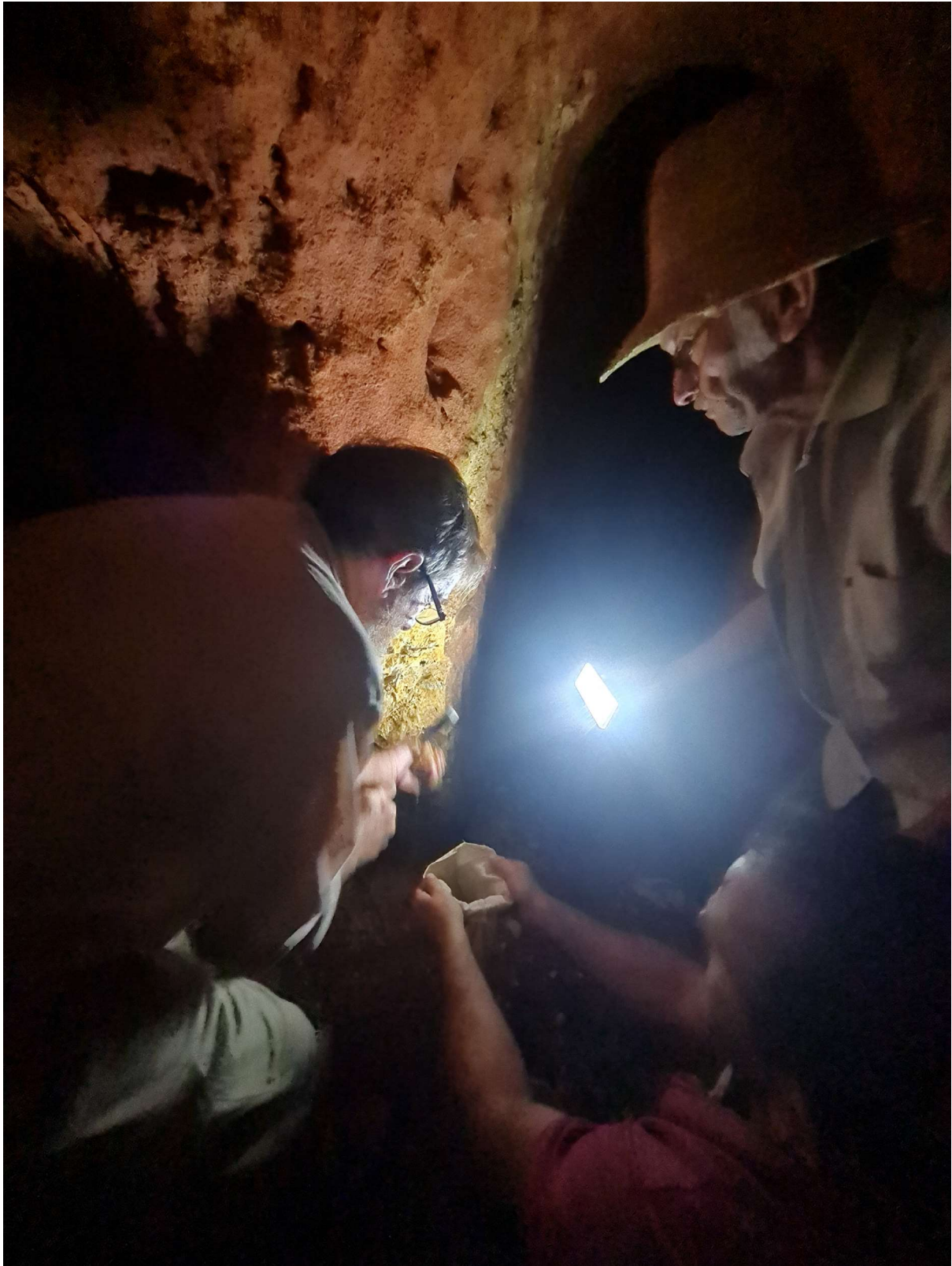
Figure 11. Small underground artisanal mine with thin pegmatites explored for gemstones in the Salinas South tenements. GMN sampled several sites in the mine in tourmaline bearing pegmatites.
