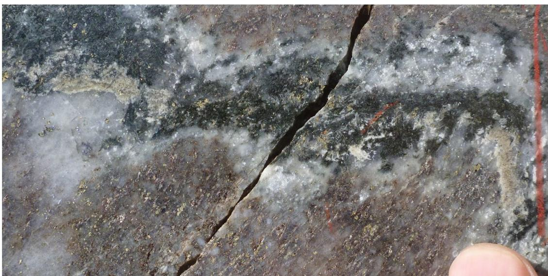
**Figure 5.** Core from CCDD002 (67.8 m) with a strongly deformed quartz-pyrite-chalcopyrite vein crosscutting well foliated and potassic altered (biotite) quartz diorite. Note the alignment of brown flakes of hydrothermal biotite and sulphide mineral within the foliation. The vein is surrounded by a zoned sodic-calcic alteration selvage consisting of dark green actinolite (inner) and greyish white albite and quartz (outer). Interval contains 0.54% Cu, 0.15 g/t Au, and 61 ppm Mo.
