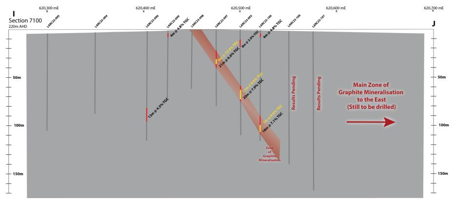
Figure 3. Section 6,317,100mN, East-West section through the Lacroma Graphite Prospect – Scale 1:1
