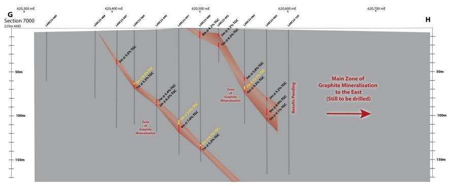
Figure 4. Section 6,317,000mN, East-West section through the Lacroma Graphite Prospect – Scale 1:1
