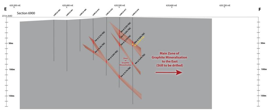
Figure 5. Section 6,316,900mN, East-West section through the Lacroma Graphite Prospect – Scale 1:1
