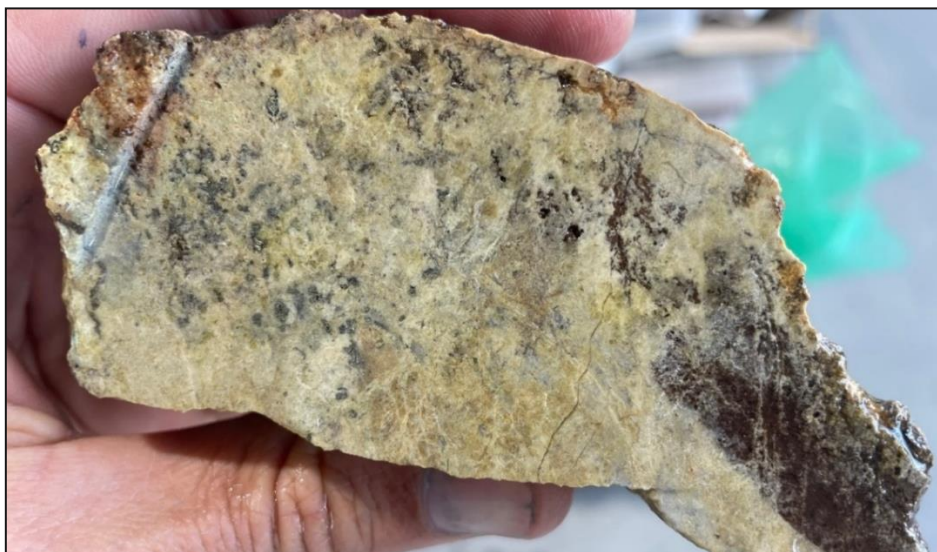
Figure 6 Yellow garnet skarn with abundant chalcopyrite and manganese oxide (black) – visual estimate 0.9% Cu
