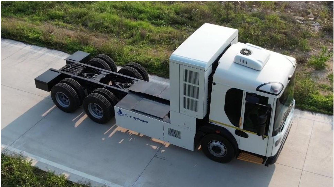
Image 1: An aerial image of Pure's first hydrogen fuel cell waste collection vehicle, which is now being fitted with refuse collection components by Bucher Municipal.
