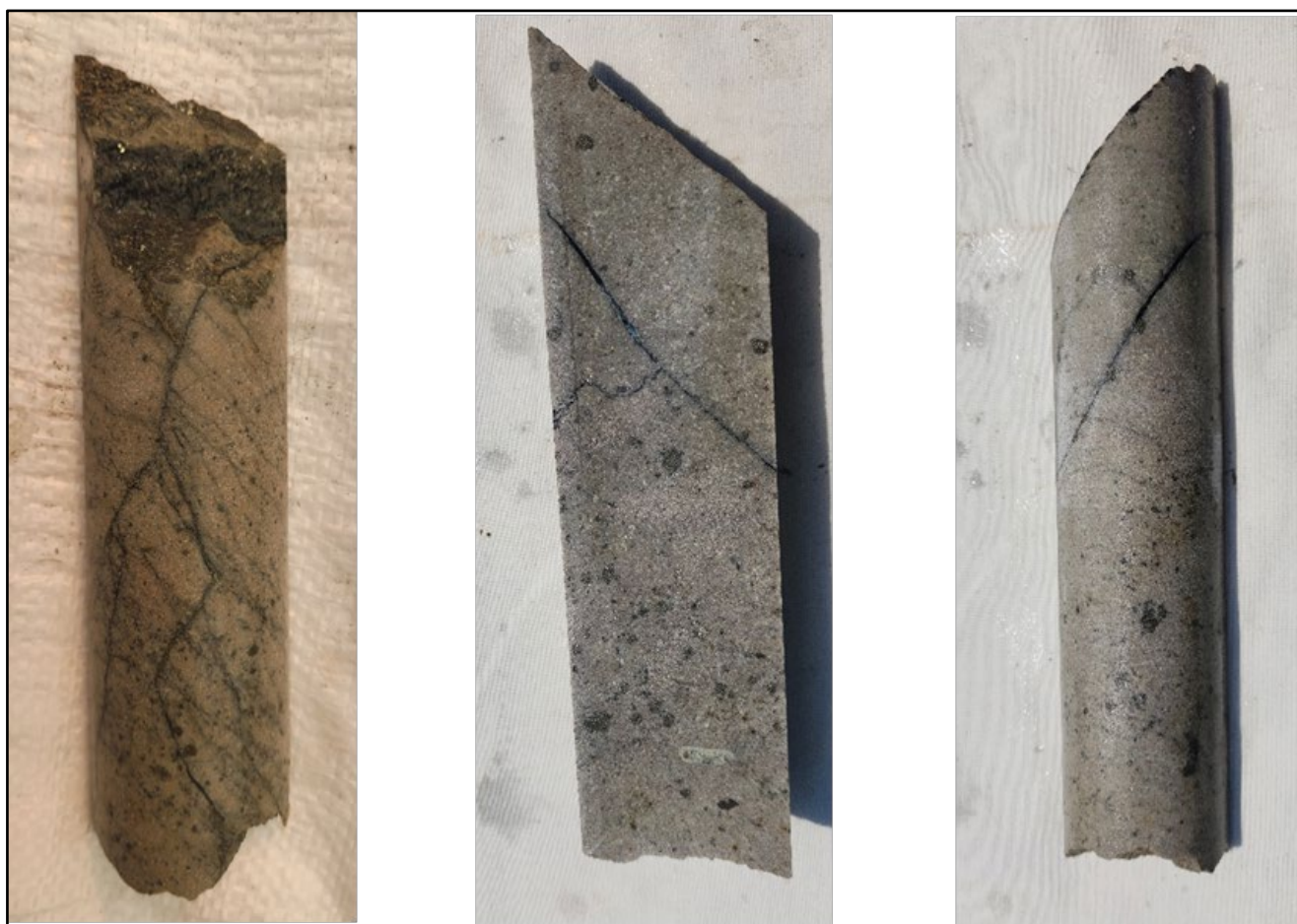
Figure 2: Examples of porphyry core from MPD005 with mineralised fractures at 346m and 399m
