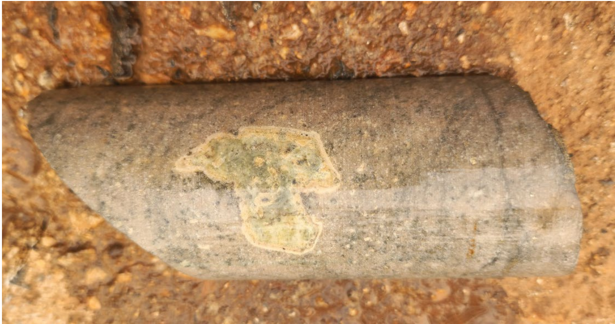
Figure 3: Epidote in sericitically altered feldspar porphyry at 342m
