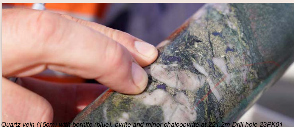
Quartz vein (15cm) with bornite (blue), pyrite and minor chalcopyrite at 221.2m Drill hole 23PK01
