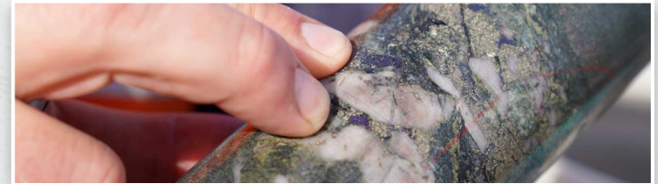
Quartz vein (15cm) with bornite (blue), pyrite and minor chalcocopyrite at 221.2m
