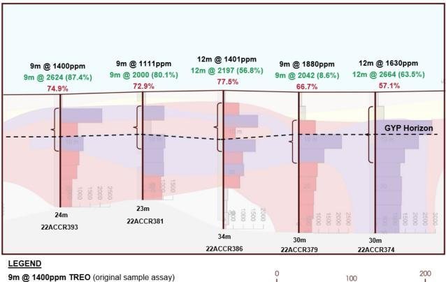
9m @ 2624ppm = 87.4% upgrade in TREO (-38µm fraction assay) 74.9% of TREO remains in -38µm fraction assay
