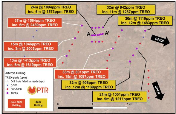
Figure 4 – Artemis Prospect – Plan view of drill collars key drill intercepts. Mineralisation currently extends over an approximate 3-kilometre trend and remains open.
