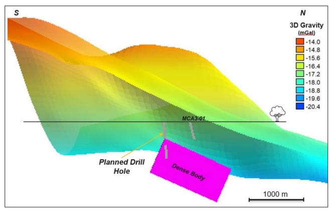
Figure 9 – 3D View looking west of the Olympus Bouguer Gravity Anomaly and dense gravity body target.
