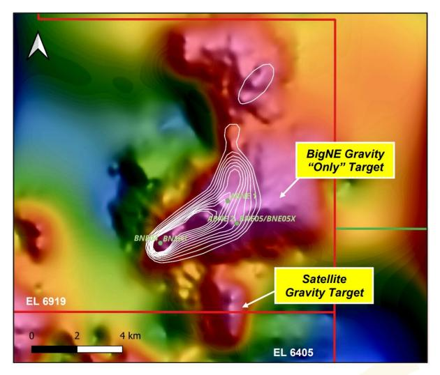
Figure 8 – BigNE and Southern Satellite Gravity Targets with high magnetic contours overlain. Note historical drilling has tested the combined magnetic and gravity responses on western half of the BigNE Target but not the gravity only target on the eastern side or satellite gravity body to the south.
