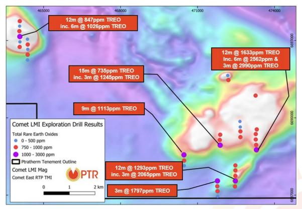
Figure 3 – Comet East – Plan view of drill collars key drill intercepts. REE's are associated with the magnetic complex. Mineralisation currently extends over an approximate 3km trend and remains open.
