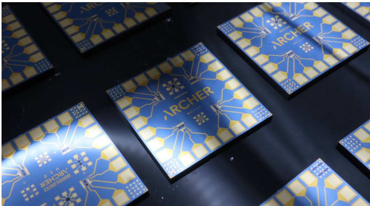
Image 2. Archer's advanced gFET chips for advanced biosensing diced from the whole four-inch wafer fabricated in a commercial foundry.
