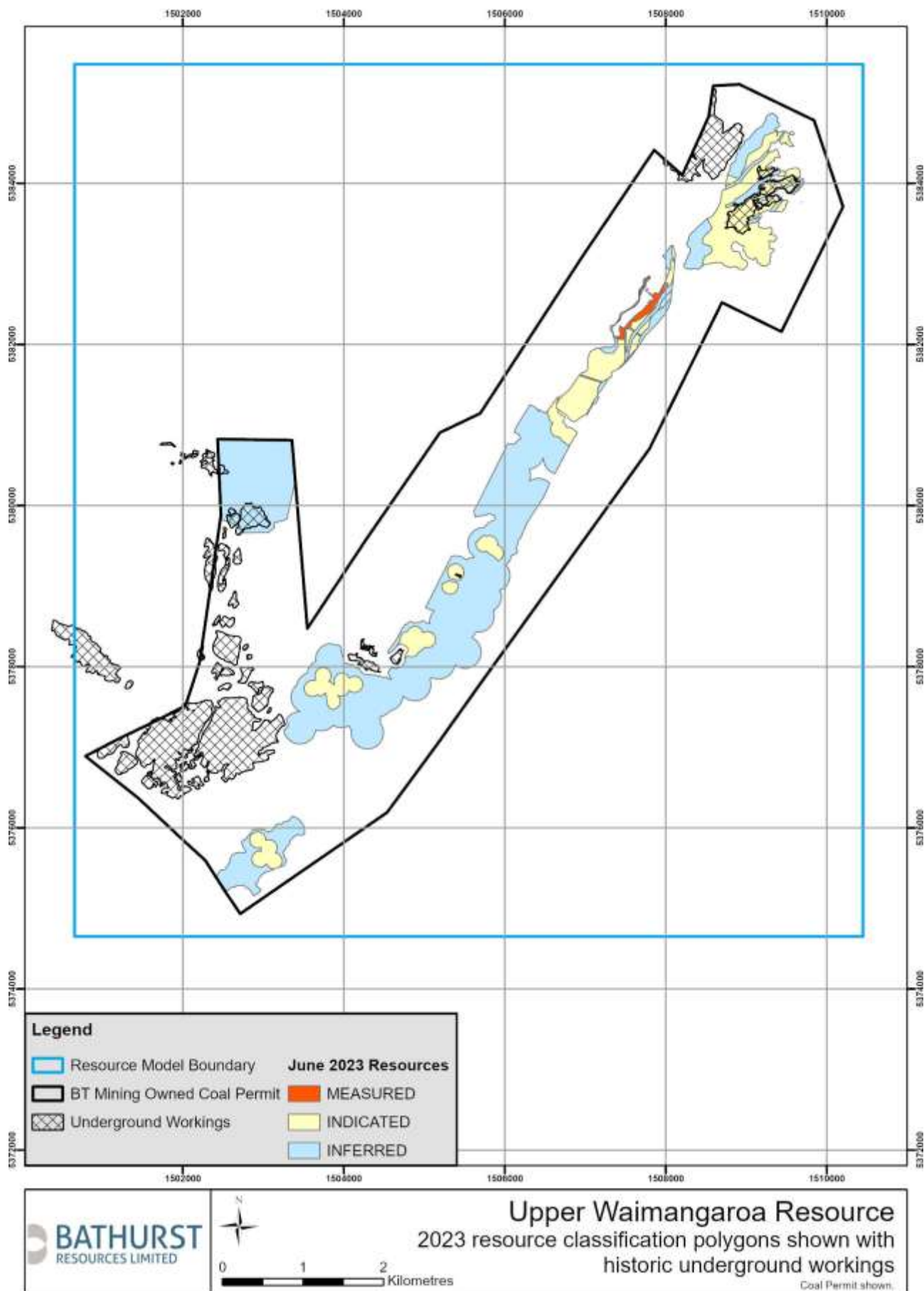
Figure 7: Extent of Underground Workings and 2023 resource classification
