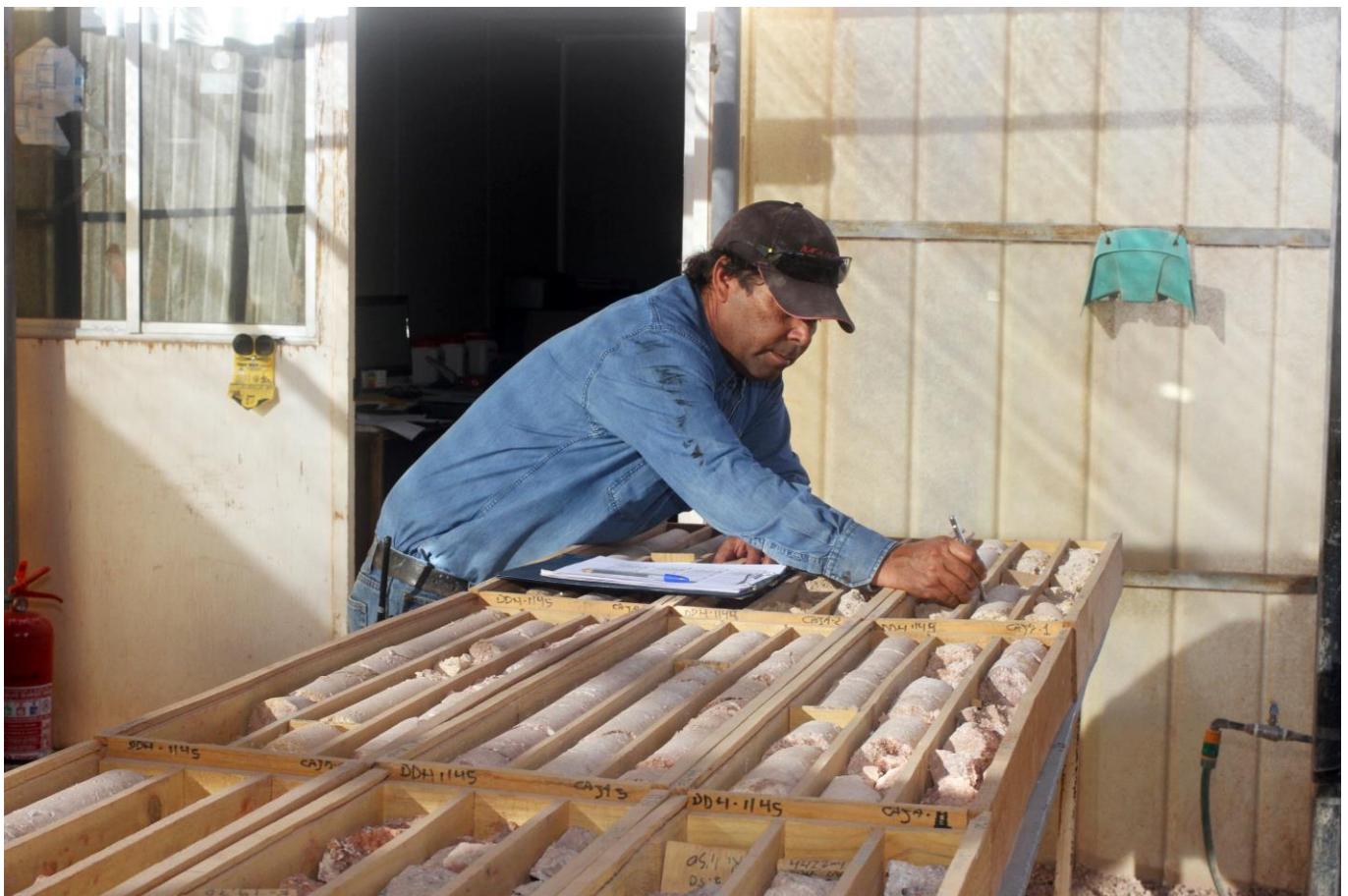
Diamond Drill Core review at Guanaco
