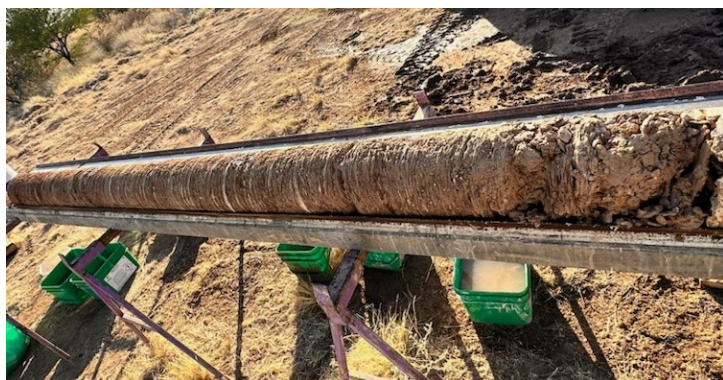
Figure 1: 8C core from 8C core trial on LIND016_B1 (twin hole)
