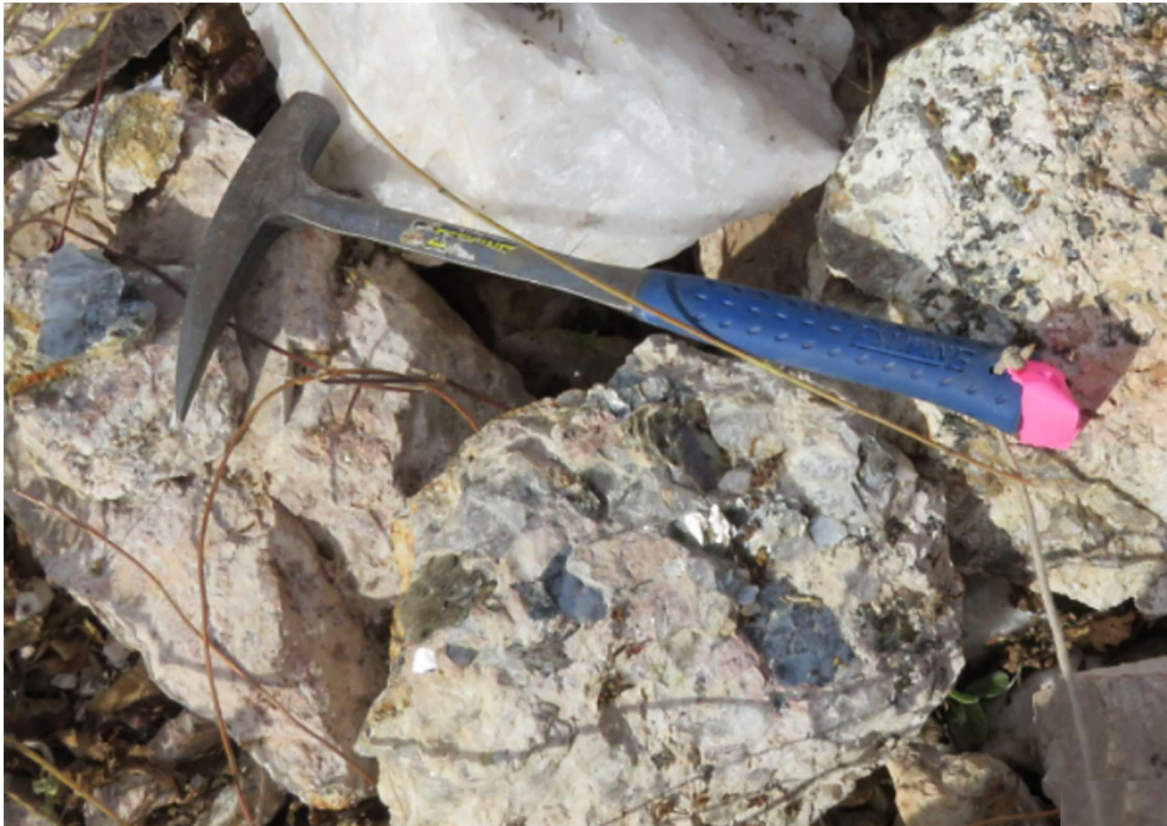
Figure 30. Range of rock types present. Quartz core material at top, left is coarse quartz-perthitic feldspar, lower centre is pegmatite with large muscovite, showing dark coloured and silver, right is fine muscovite in quartz feldspar pegmatite.
