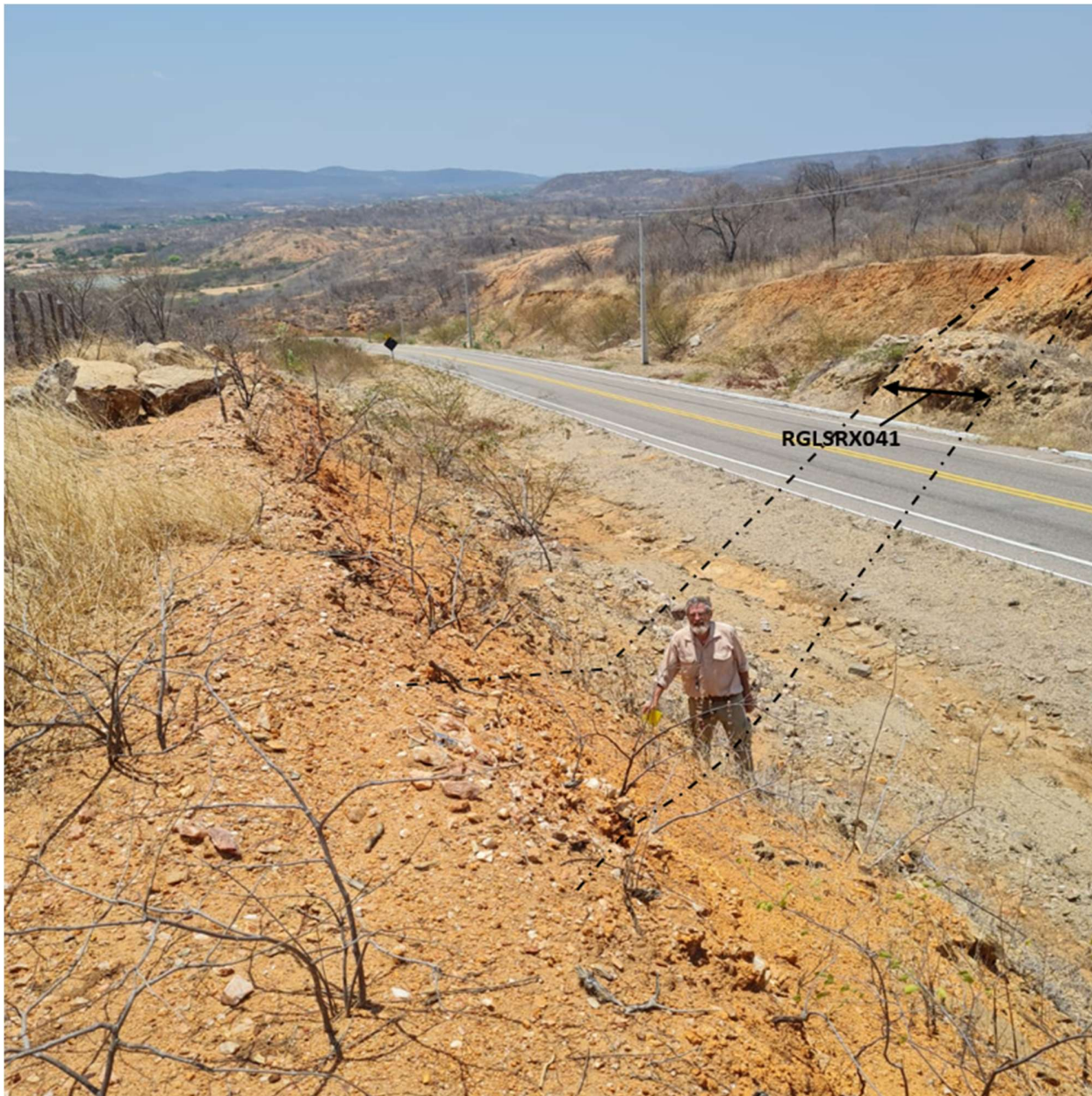
Figure 22. Photo of the 6 m wide pegmatite sampled in the road cut that is not visually detectable at surface.
