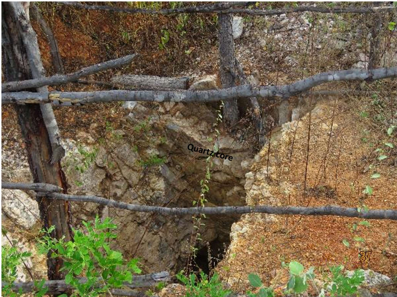
Figure 29. Artisanal mine for beryl in a coarse grained pegmatite with a quartz core.
