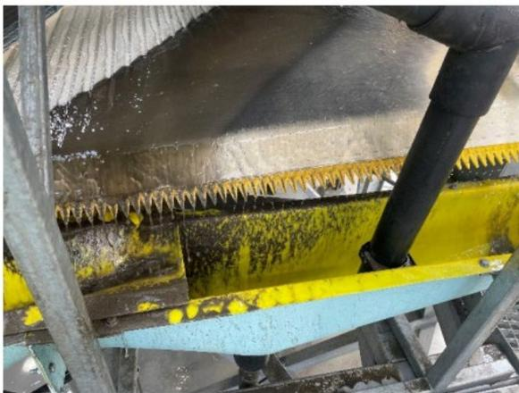
*Figure 7 – Tungsten separation on shaking tables*
