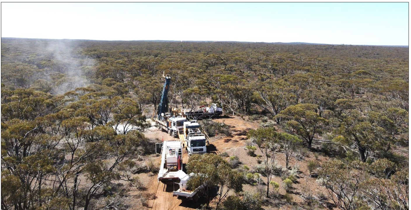
Figure 2 – Reverse Circulation Drilling at the Lefroy Lithium Project.
