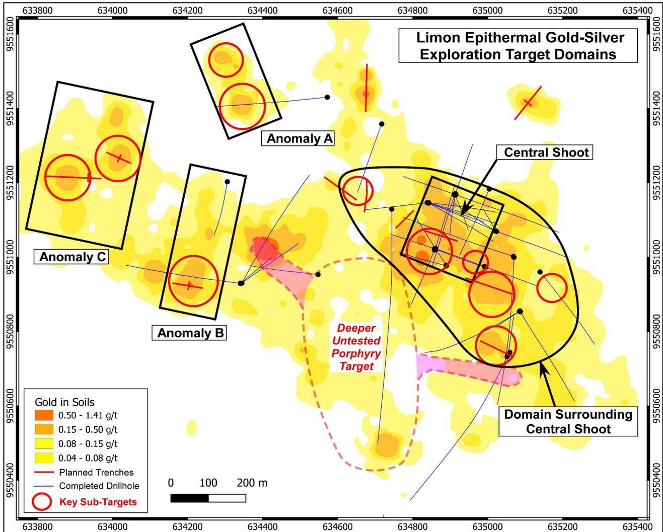
**Figure 1:** Limon gold in soils map showing extensive anomalous gold over an area of 1.7km x 700m. The black outlined areas are those referred to in Table 1 and form the basis of the Exploration Target. Red circled areas are key sub-targets. The red dashed line shows the deeper Limon porphyry target outline with fingers that extend to surface to the NW and the East. Follow-up exploration activities are discussed in the text.
