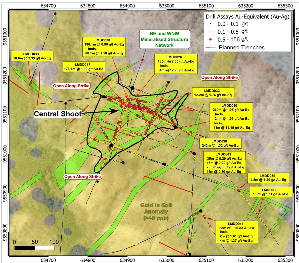
**Figure 2:** Limon epithermal gold-silver system in plan view, showing multiple mineralised structures in green. High-grade domains are at intersections of NE and WNW trending structures. Several additional targets have been defined based on gold-in soil and zinc-in-soil anomalies, and structural interpretation and follow-up drilling will be undertaken on these targets in 2024. See Figure 1 for a broader context within the very large Limon target area.
