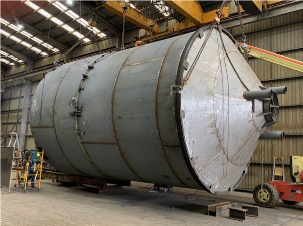
Figure: Spray Roaster reactor vessel workshop fabrication complete
