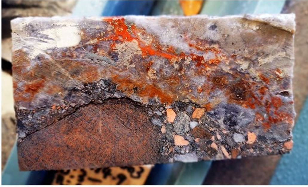
*Figure 1. Quartz-siderite-pyrite-chalcopyrite breccia hosted vein from diamond drill core at the Benmara Copper Project (23BNM003: 174.8m, <0.1% Cu)*
