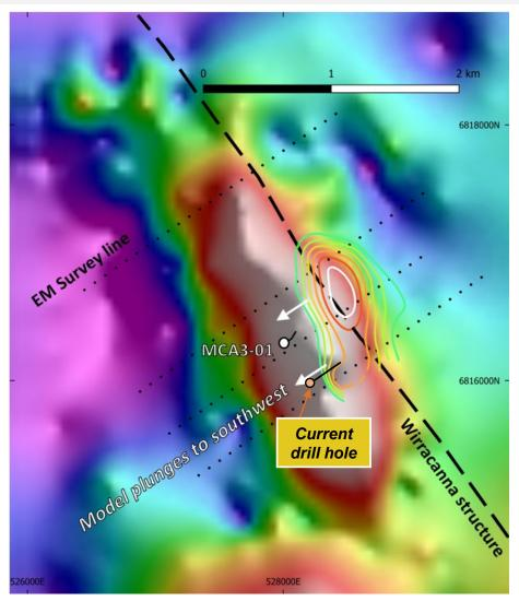
**Olympus Geophysical Response -** 1VD Bouguer Gravity Image overlain by late time EM contours showing the position of the top of the conductive plate on the eastern flank of the gravity body which plunges steeply back to the southwest.
